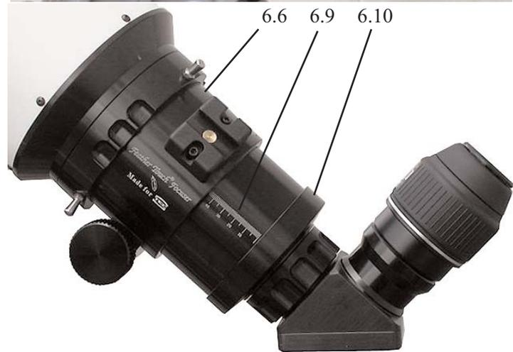
**NOTE: It is possible to reverse the pinion assembly for left handed preference but Starlight Instruments does not recommend the user reversing this assembly because of possible misalignment resulting in a loss of performance or possible damage.**
