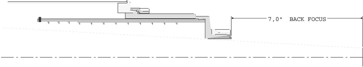
Focusing tube is completely "OUT"
