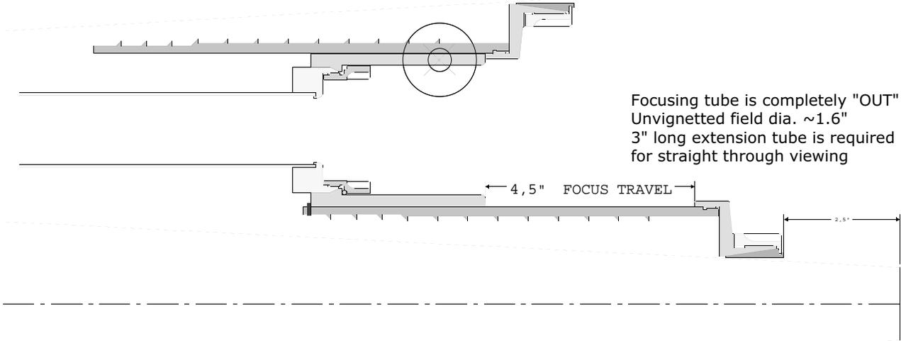
With the 2" diagonal focusing tube is in the middle position
