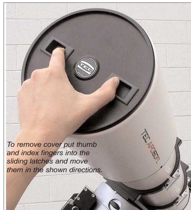
*To remove cover put thumb and index fingers into the sliding latches and move them in the shown directions.*
