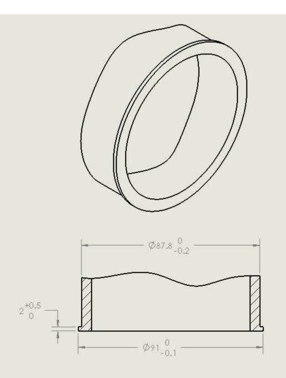
FRC ADAPTER sample for using standard threaded ring
