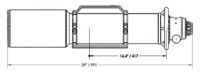
Length in working position with the focuser in the middle of focusing range Approximate CoG position from the middle of wheel and 2.5lb /1kg load
