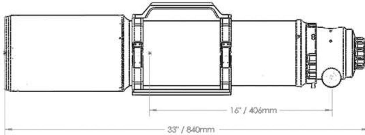
Length in working position with the focuser in the middle of focusing range 43" / 1090mm
